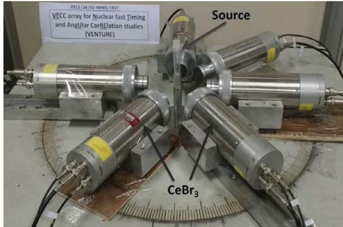
Figure 4.11: Stand alone setup of VENTURE array with six  $\text{CeBr}_3$  detectors which are arranged on angular correlation table (discussed in Section 5.3 of Chapter 5).
