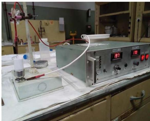
Figure 6.4: The experimental setup of electrodeposition technique used, in the present thesis work, for preparation of targets is shown. The figure has been taken from Ref. [SAH18a].
