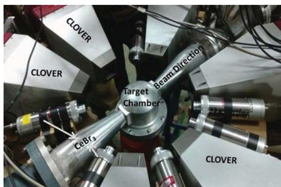
Figure 9.2: In-beam setup of VENTURE array of six  $\text{CeBr}_3$  detectors coupled to VENUS array of six Clover detectors is shown.
