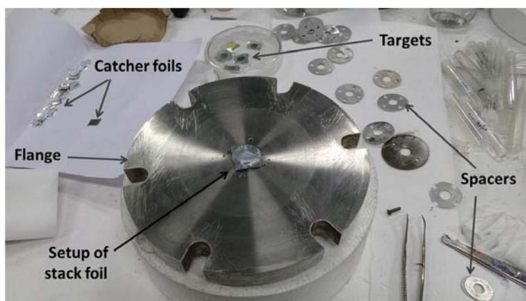
Figure 6.6: The snapshot of the flange and the preparation of stacked foil on it.
