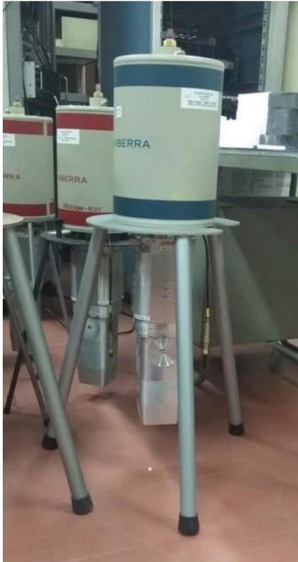
Figure 3.2: Picture of a Clover detector used for the experiments in the present thesis.
