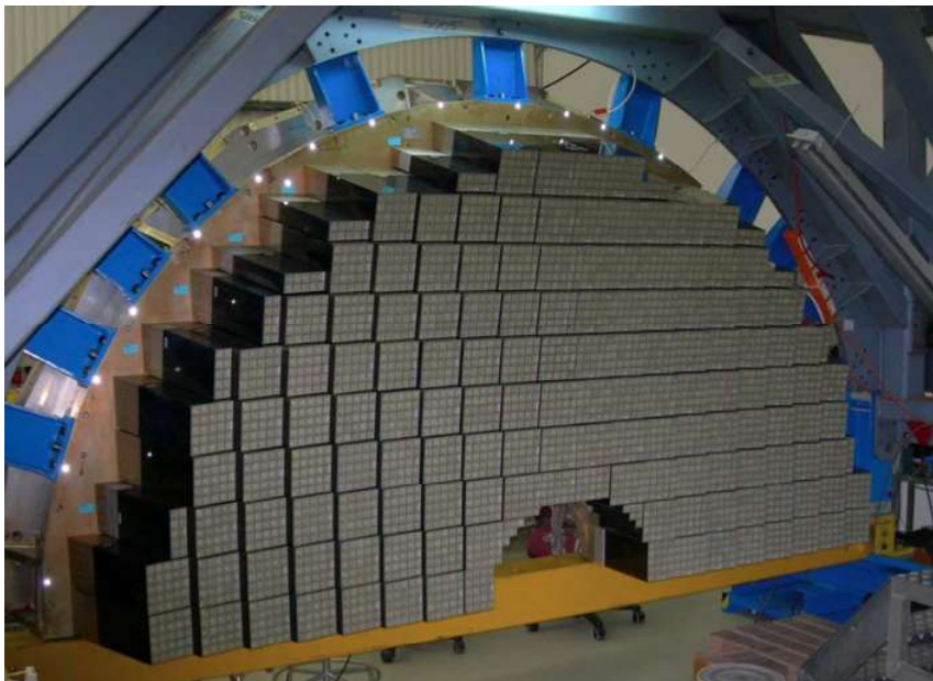
Figure 3.8: An endcap Dee, fully equipped with supercrystals [67].
