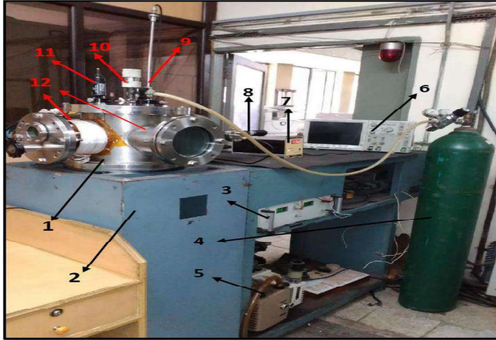
Figure 2.3: Picture of the dc glow discharge plasma device: 1) Vacuum chamber, 2) Stand, 3) High voltage power supply, 4) Argon gas cylinder, 5) Rotary pump, 6) Digital oscilloscope, 7) Pressure reading meter, 8) Langmuir probe, 9) Power supply connection, 10) Pressure control unit: needle valve, 11) Pirani gauge, and 12) Side cylindrical chambers attached with main vacuum chamber
