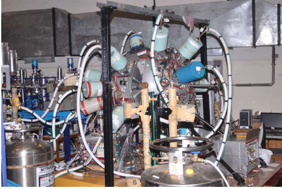
Figure 3.2: The INGA array of Compton suppressed clover detectors set up at TIFR. Figure taken from Ref. [58].
