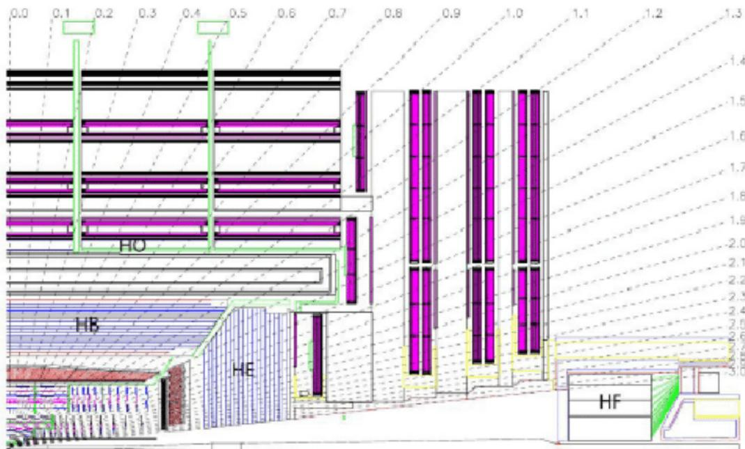
Figure 3.15: A longitudinal view of one quarter of the CMS detector in the  $r-\eta$  plane. The layout shown is up-to the HCAL indicating the components of the HCAL: hadron barrel (HB), hadron outer (HO), hadron endcap (HE) and hadron forward (HF)
