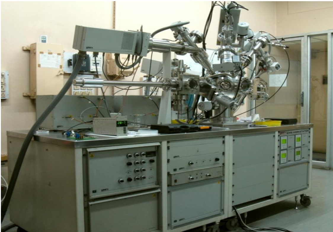
Figure 5.10: Image of the SIMS instrument used for calculating the composition profile of the rare-earth based LB films at Saha Institute of Nuclear Physics, Kolkata, India.
