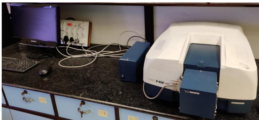
Figure 2.14: *Photograph of the UV-vis-NIR spectrophotometer.*
