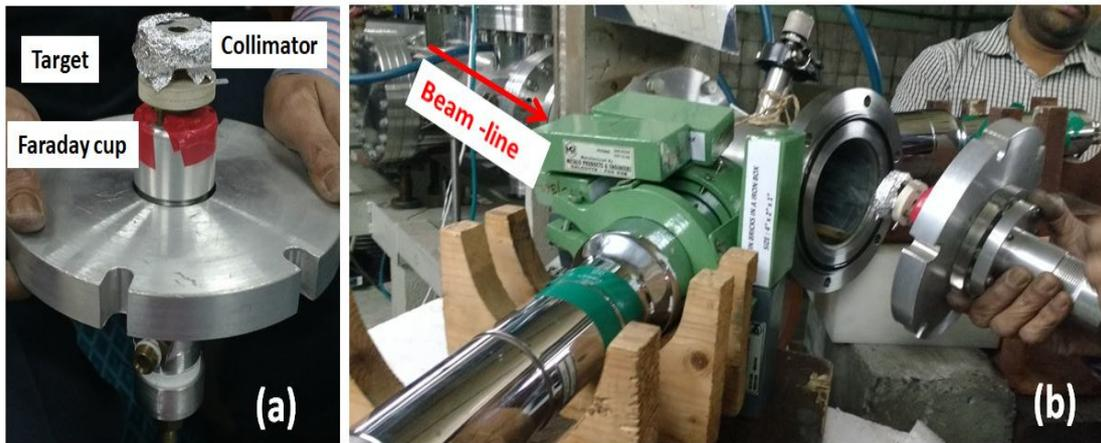
**Figure 2.4:** (a) The collimator, target holder, and the Faraday cup as indicated in the picture constitute the irradiation flange. (b) The flange position and the direction of the beam along with the beamline are marked in the picture.
