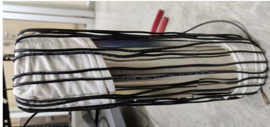
**Figure 2.10:** One of the home-made cylindrical  $\mu$ -metal shields. The black wire was wrapped in the cylinder with toroidal fashion for the degaussing process.
