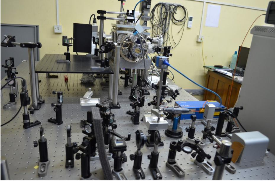
**Figure D.10:** An image of the MOT setup in our laboratory.
