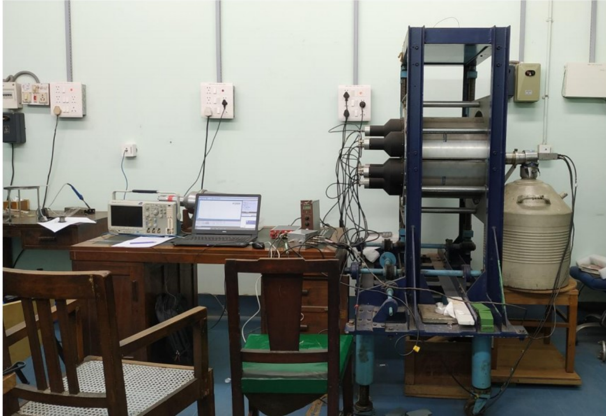
Figure 8.5: The shielding arrangements at Lab II with SUM spectrometer for the same 20% relative efficiency HPGe detector. The empty space in the SUM spectrometer borehole has been blocked with Pb blocks from one end and the HPGe detector is inserted from the other end.
