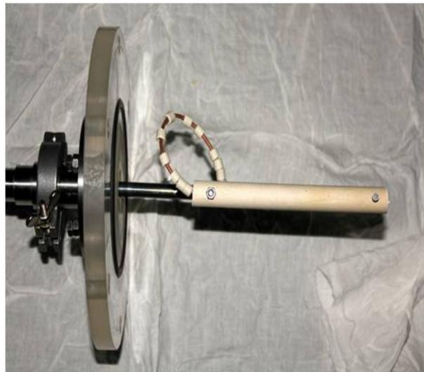
*Figure 3.14 Picture of the wall probe for DC bias measurement.*
