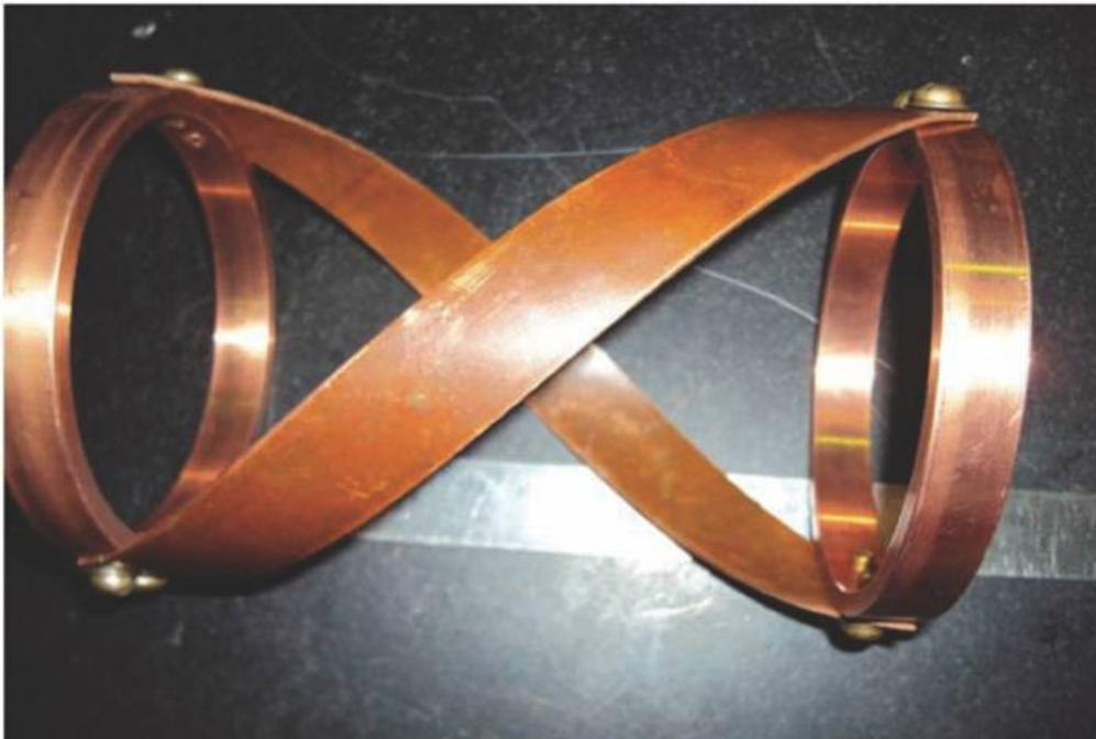
*Figure 3.5 Picture of the half helical  $m=+1$  antenna just before installation.*
