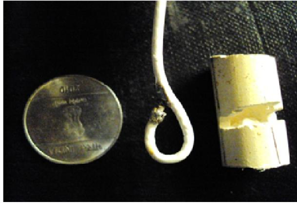
*Figure 3.30 Picture of the single loop B-dot probe made of a coaxial cable.*
