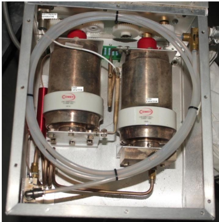
*Figure 3.4 Picture of the inside of the match box showing the variable Load and Tune Capacitors with auxiliary inductors.*
