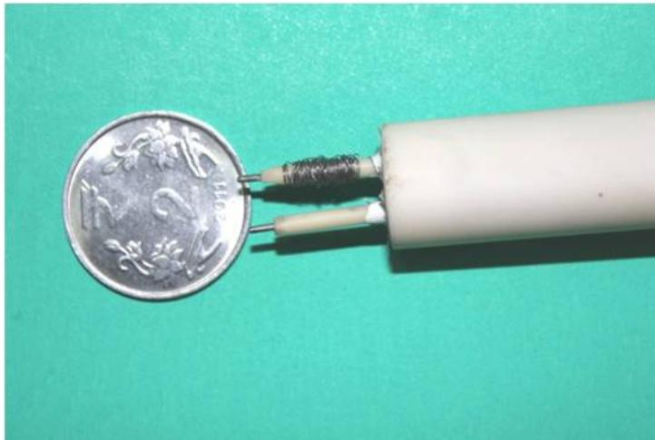
*Figure 3.15 Picture of the RF compensated probe along with an uncompensated probe.*
