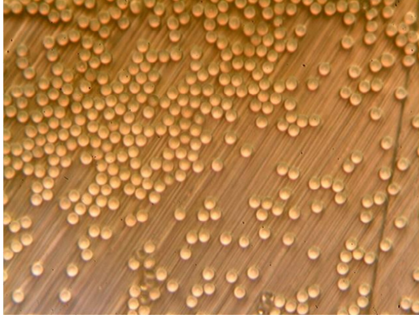
Figure 2.4: The image of a sample of melamine formaldehyde (MF) condensation resin particles being used in experiments having average diameter as 6.48\ \mu\text{m} , obtained using a microscopic shows that the dust particle are spherical in nature (to a very good approximation). The size distribution is extremely narrow (standard deviation is 0.1\ \mu\text{m} ).
