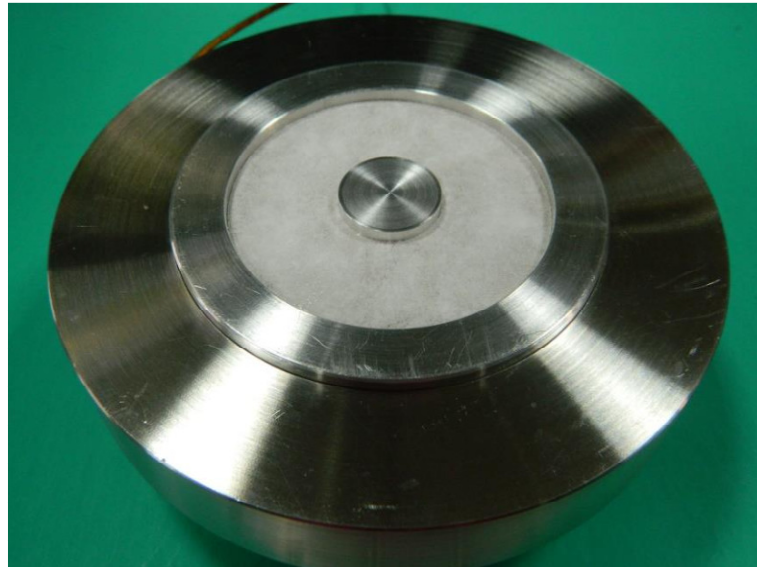
Figure 5.1: The picture shows the concentric metallic disk placed on the cathode surface along with the concentric metallic ring. The annular region between the ring and disk is covered by MF dust particles.
