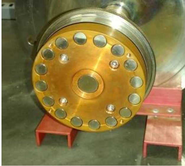
Figure 3.4: Photograph of the magnets arranged in the copper housing.
