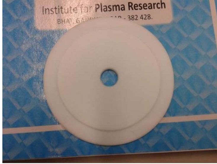
Figure 6.6: The photograph of actual anode stop, it is mounted on the surface of the anode, the peripheral region is hence blocked from the plasma
