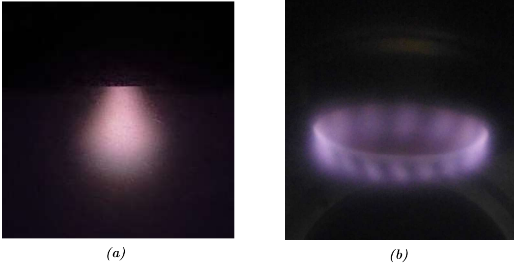
Figure 5.1: Images of (a) C-Mode ( 3 \times 10^{-2} mbar) and (b) P-Mode discharge ( 8 \times 10^{-2} mbar).
