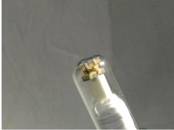
**Fig. 2.6.** Photograph of designed B-dot probe
