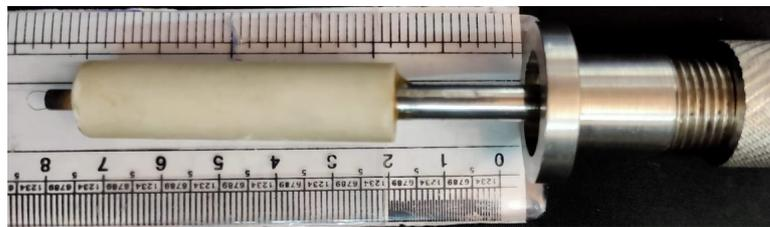
Figure 2.5: A photograph of emissive probe used in the experiments.
