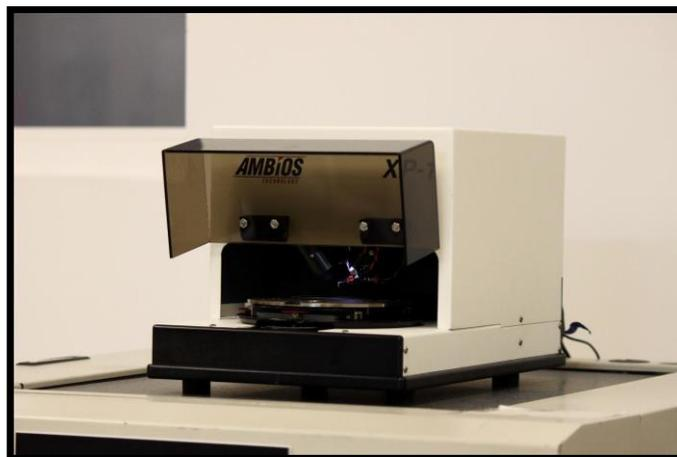
Figure 2.6: Stylus surface profilometer.
