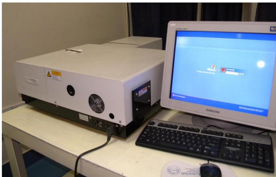
Figure 2.15: UV-Vis spectrophotometer
