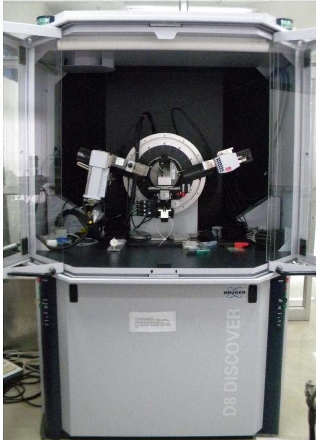
Figure 2.13: XRD setup
