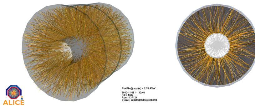
Figure 2.9: (Color online) Event display of the tracks reconstructed inside TPC in Pb-Pb collisions at  $\sqrt{s_{NN}} = 2.76$  TeV during 2010.
