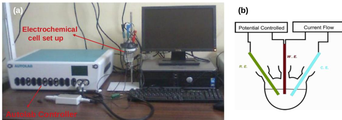
Figure 2.6: (a) PGSTAT 302N Autolab electrochemical workstation with a chemical cell set up and (b) Schematic diagram of the electrode arrangement within the chemical cell.
