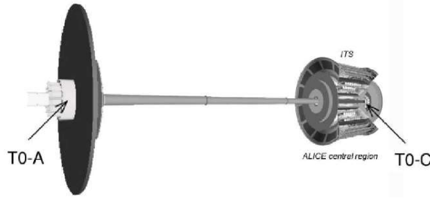
Figure 2.8: Position of the T0 detector inside ALICE experiment [16].
